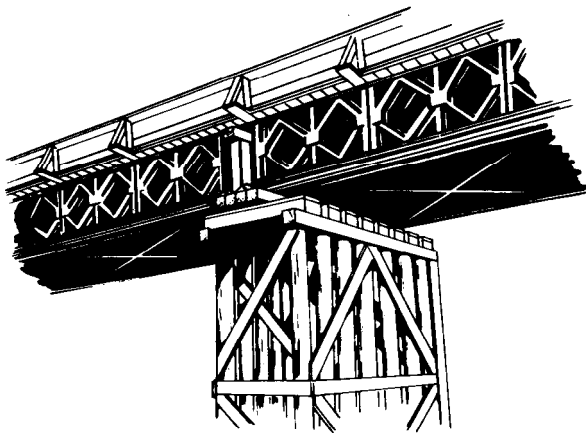
Figure 12-5 Junction of two deck spans on an intermediate pier; timber bent supports the decking between ends of span
